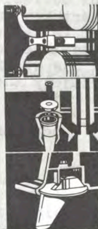
Sacrificial anodes in critical areas are designed to attract corrosion, so the rest of the motor won't.
